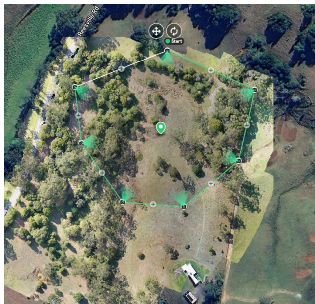
Figures 4 & 5 Drone deploy software is utilised to monitor the project site providing repeatable imagery over time and establishing photo monitoring points.
