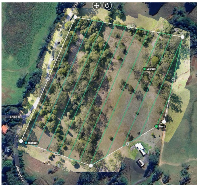
Figures 4 & 5 Drone deploy software is utilised to monitor the project site providing repeatable imagery over time and establishing photo monitoring points.
