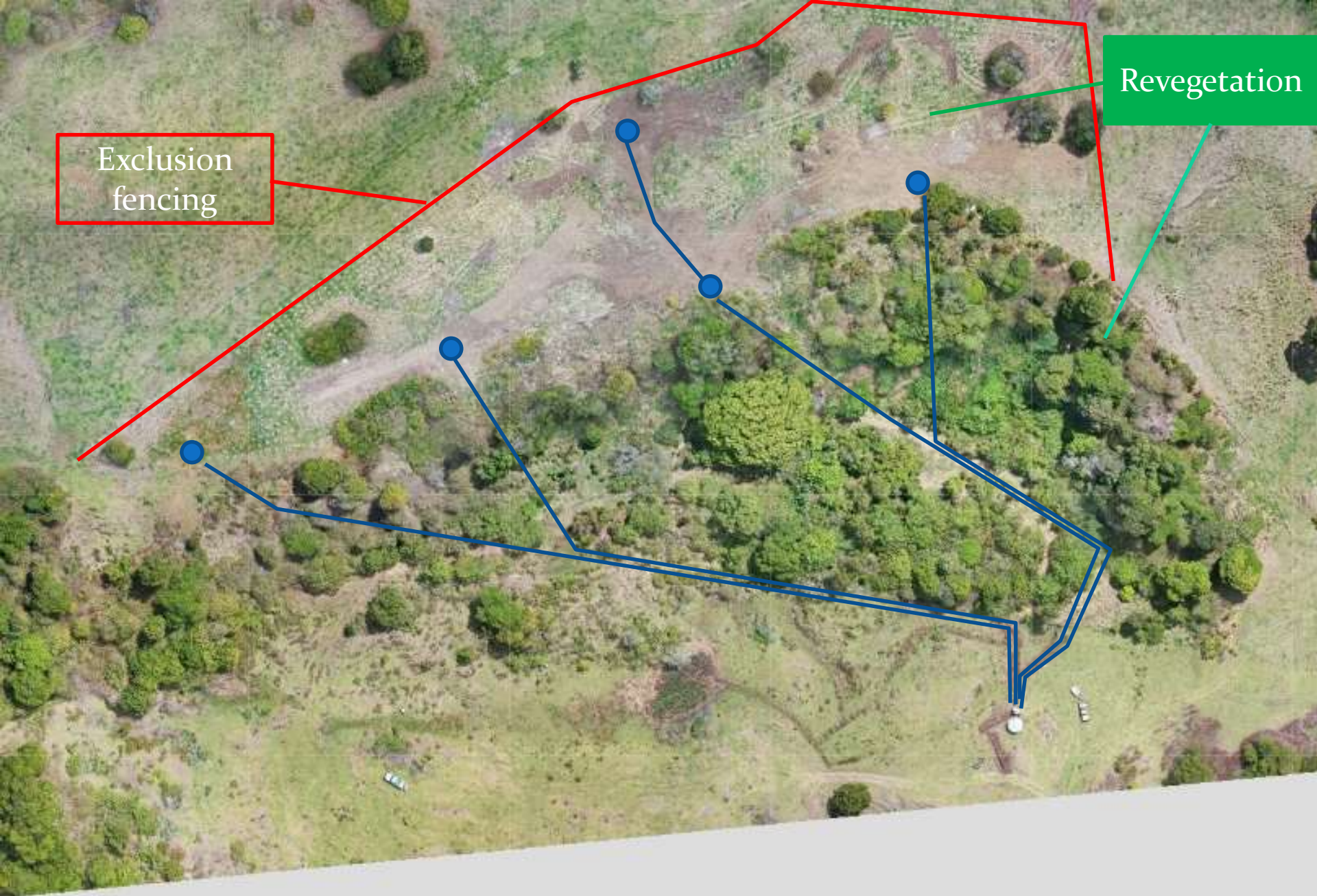
5 Drainage wells installed and fitted with poly pipe which then feeds into a header tank and then out into two troughs for cattle.
