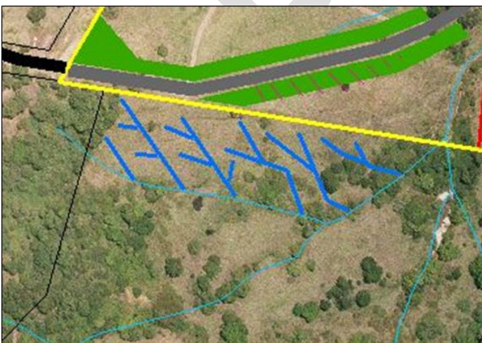
Above: Google image from June 2007 clearly showing the drainage line from the Ferriday property into the Ling property and cutting down the eastern landslip.
